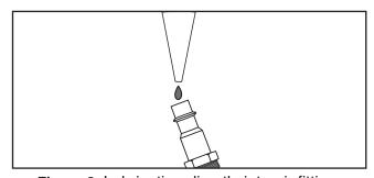
Figure 3. Lubricating directly into air fitting.
